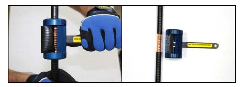
Step 4 Continue to rotate ground kit tool until jacket cuts free
