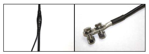
Step 9 Apply three overlapping layers of vinyl electrical tape extending 2" beyond the butyl mastic Step 10 Attach lug and heat shrink sleeve, and bolt the lug into position using the appropriate hardware
